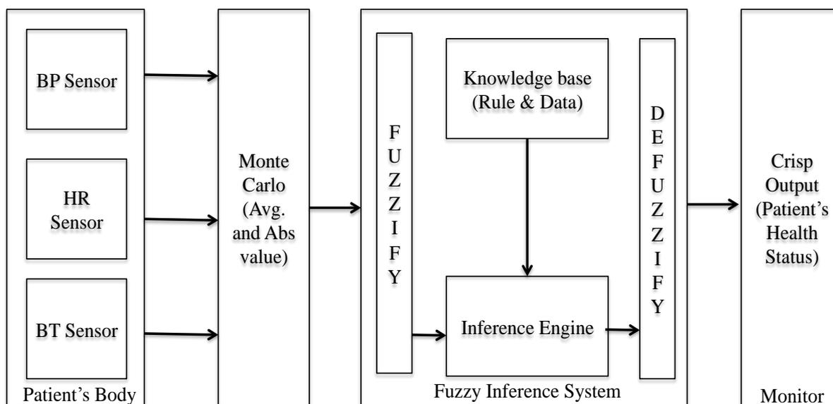
Figure 1 : Architecture of Fuzzy based Multisensor data fusion system.
