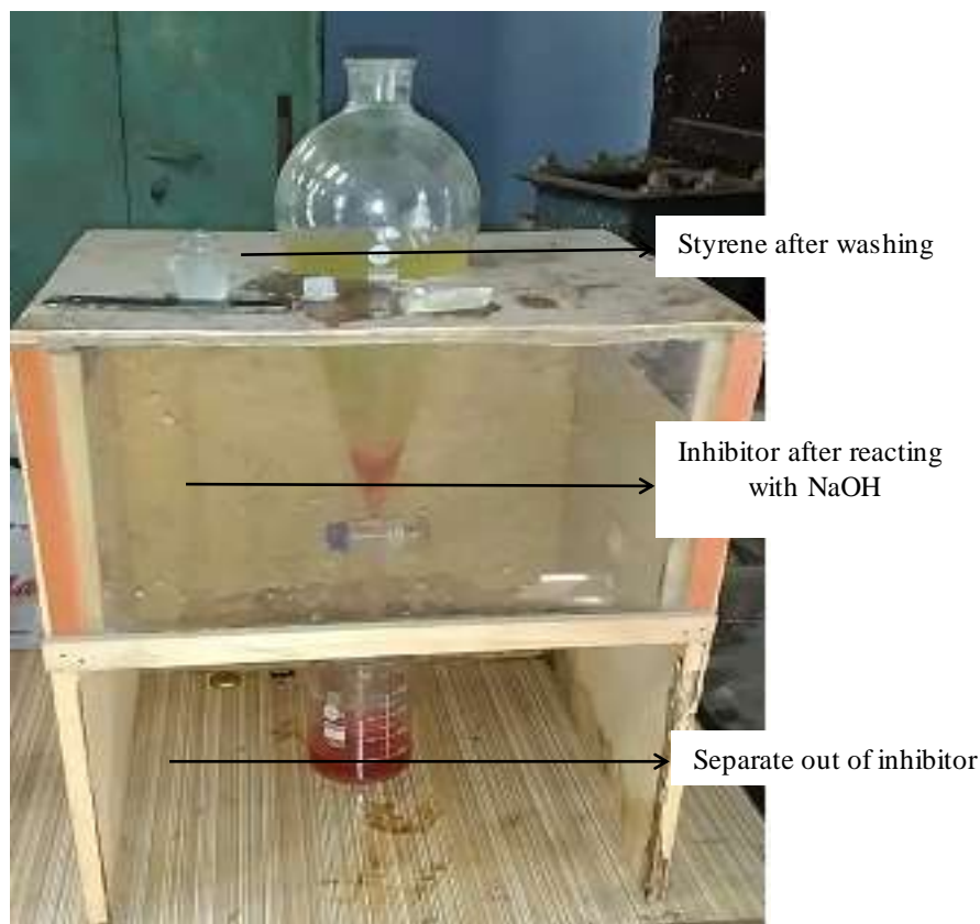
Figure 2 Washing of styrene by NaOH
