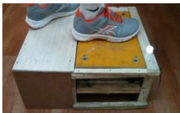
Figure 6: LED Glows when a person step on the platform
