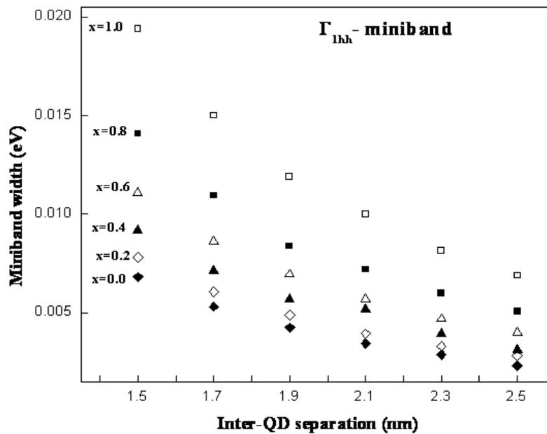
Figure 2. The  $\Gamma_1$  - mini band width as calculated for the heavy holes versus the inter-QD separation for different Zn compositions.
