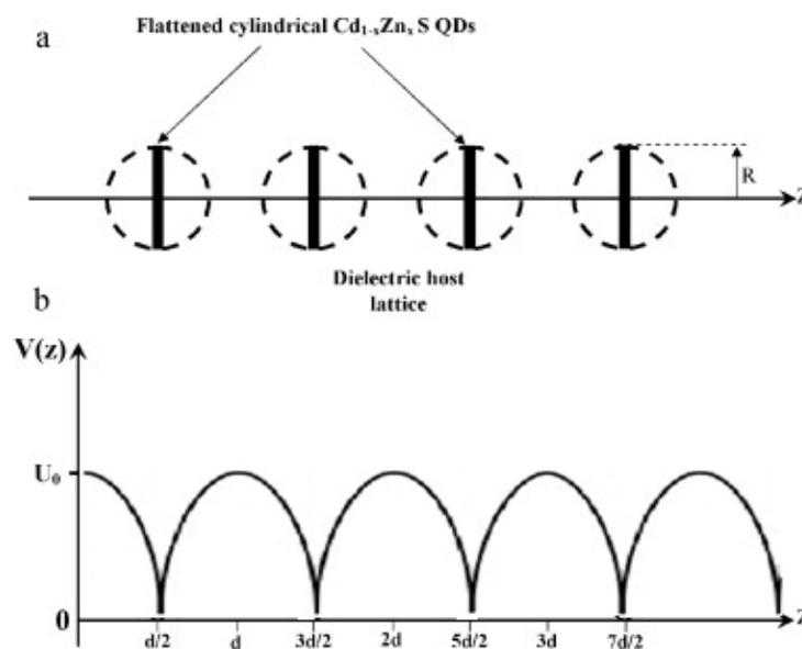
Figure-1(a): A schematic diagram of  $Cd_{1-x}Zn_xS$  QD super lattices according to the flattened cylindrical geometry – (b) The barrier potential in the framework of the novel potential model.
