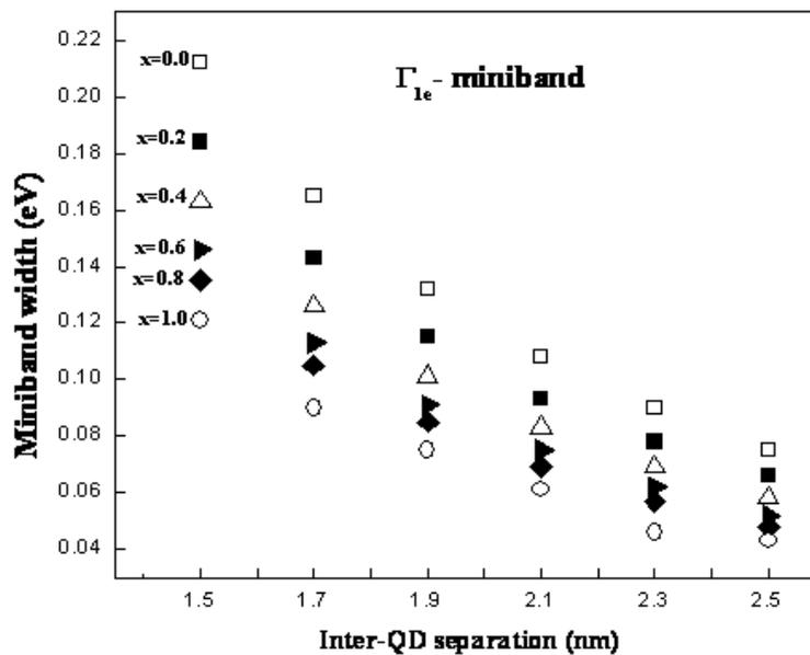
Figure 4. The  $\Gamma_1$ -mini band width, as calculated for electrons versus the inter-QD separation for different zinc compositions [29].
