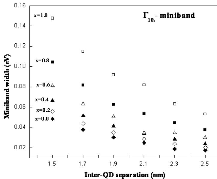
Figure 3. The  $\Gamma_1$  - mini band width as calculated for the light holes versus the inter-QD separation for different Zn compositions.
