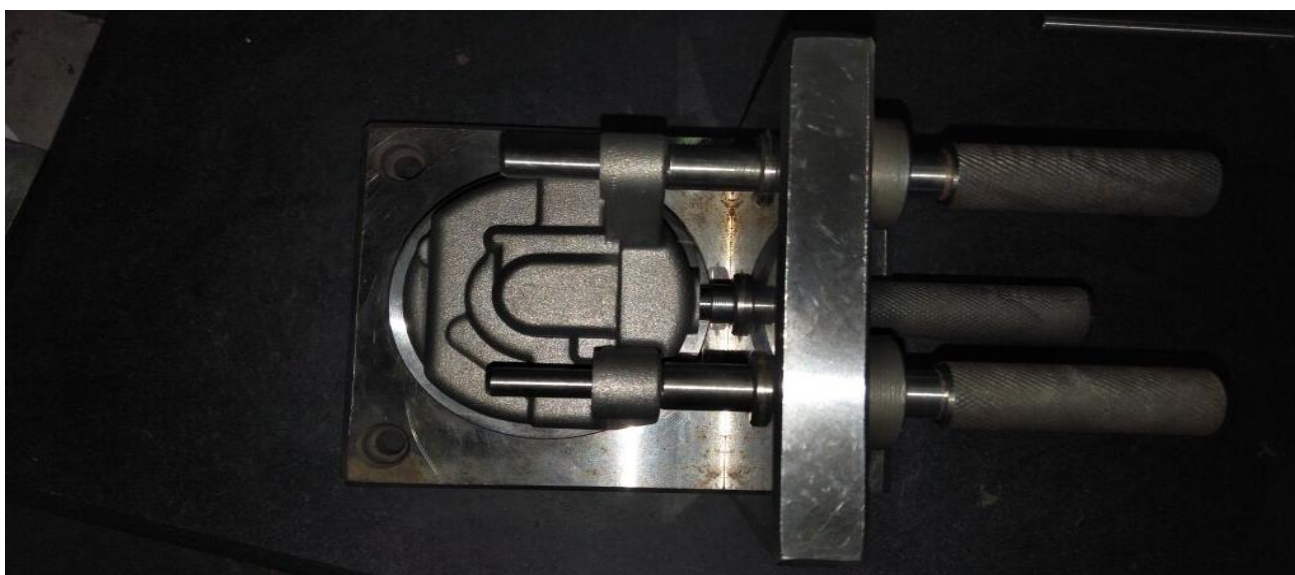
Fig.3:- Top view of Inspection Gauge with Component
