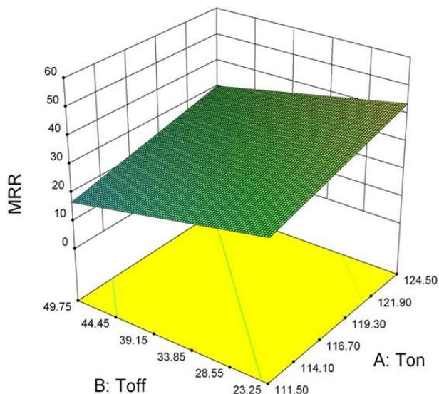
Figure 5: 3-D graph of Effects of Ton and Toff on MRR
