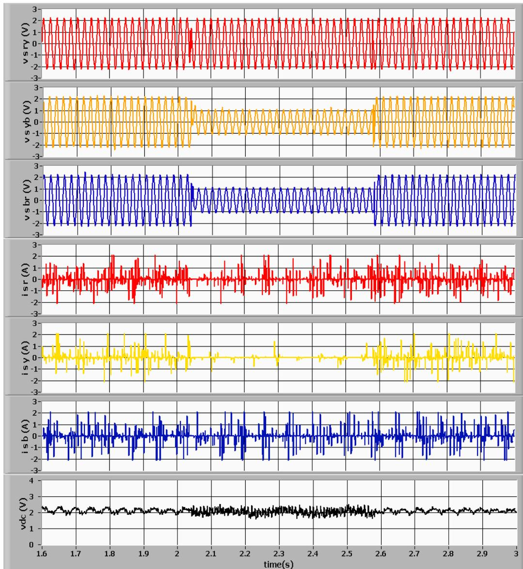
Figure 8. Experimental results showing three-phase source voltages, currents and DC-Link voltage during SLG fault (Type-B) with supercapacitor as ride-through alternative. Voltage scale: 100 V per division. Current scale: 2.25 A per division. DC-Link Voltage scale: 100 V per division.
