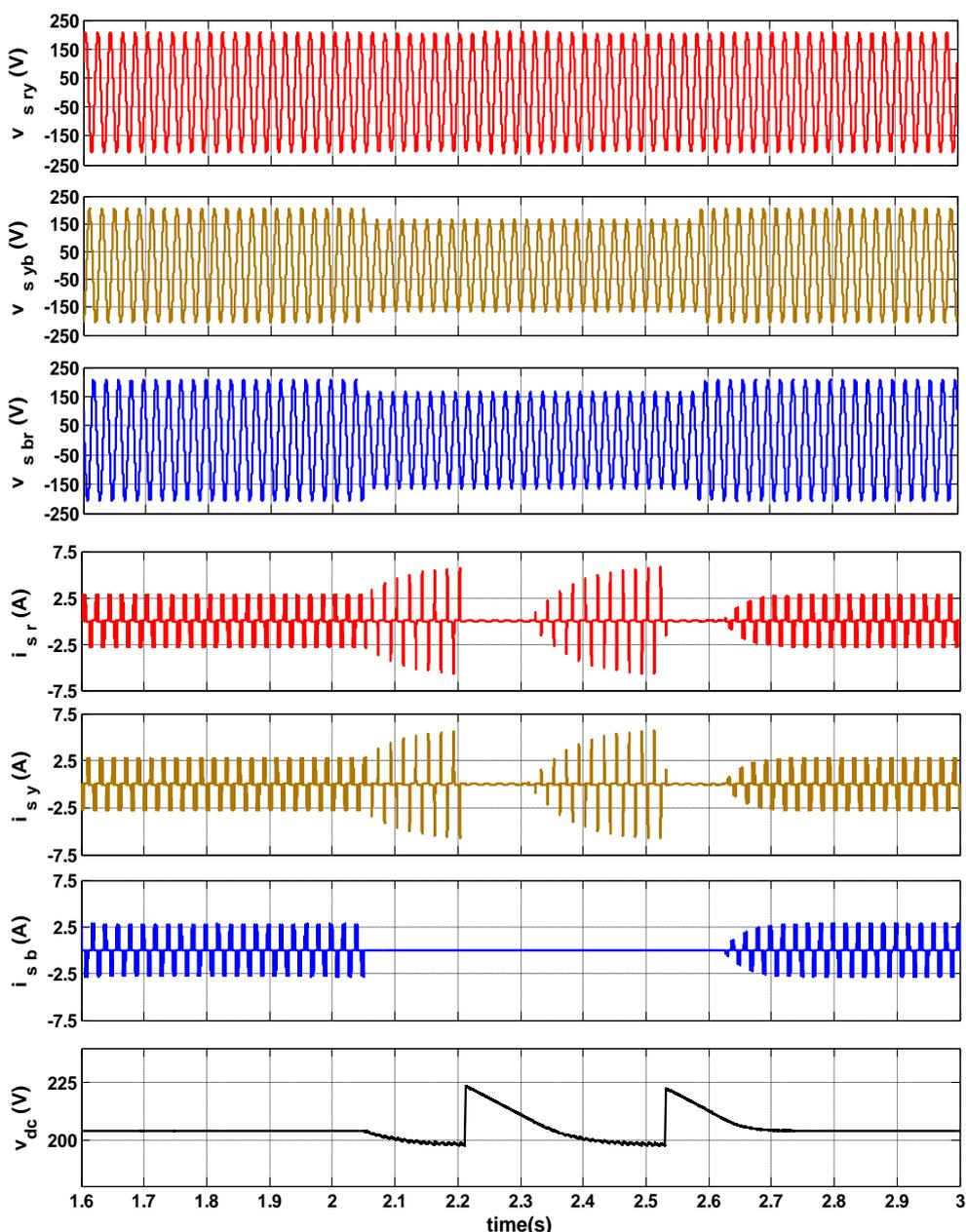
Figure 7. Simulation results showing three-phase source voltages, currents and DC-Link voltage during SLG fault (Type-B) with supercapacitor as ride-through alternative.
