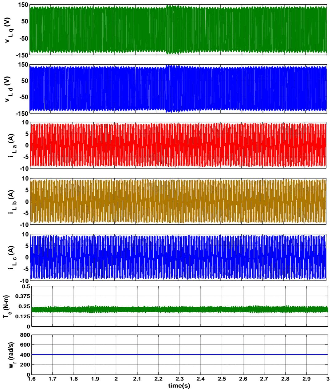
Figure 9. Simulation results showing stator voltages in d-q frame, three-phase stator currents, electromagnetic torque and rotor speed during SLG fault (Type-B) with supercapacitor as ride-through alternative
