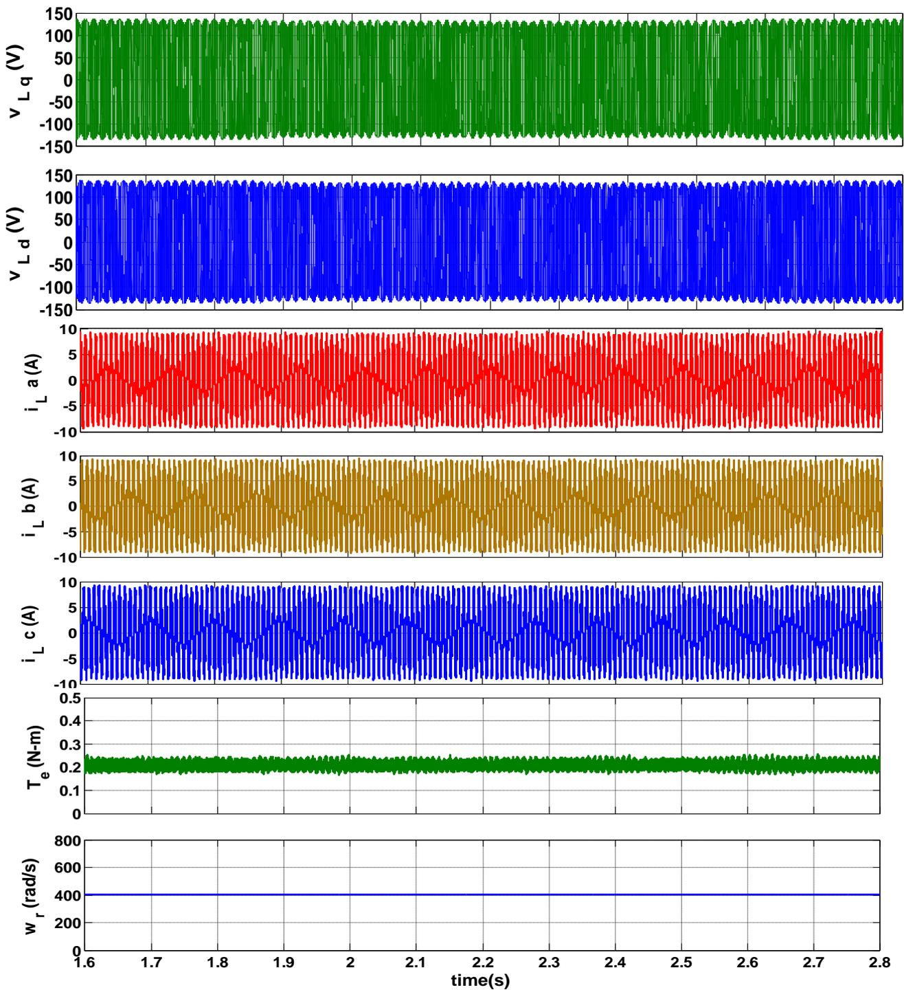
Figure 5. Simulation results showing stator voltages in d-q frame, three-phase stator Currents, electromagnetic torque and rotor speed during SLG without any ride-through.
