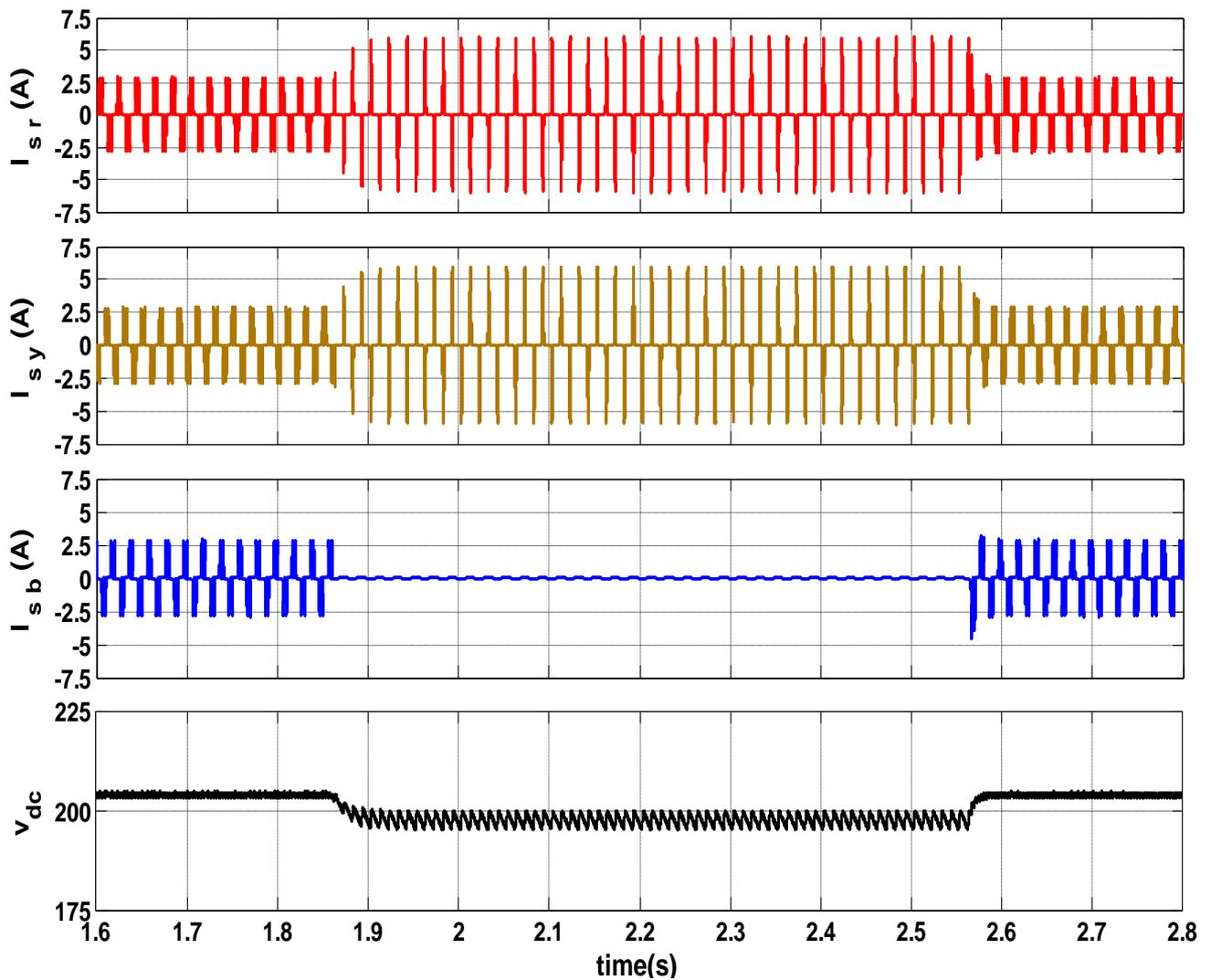
Figure 3. Simulation results showing three-phase source voltages, currents and DC-Link voltage during SLG fault (Type-B) without any ride-through.
