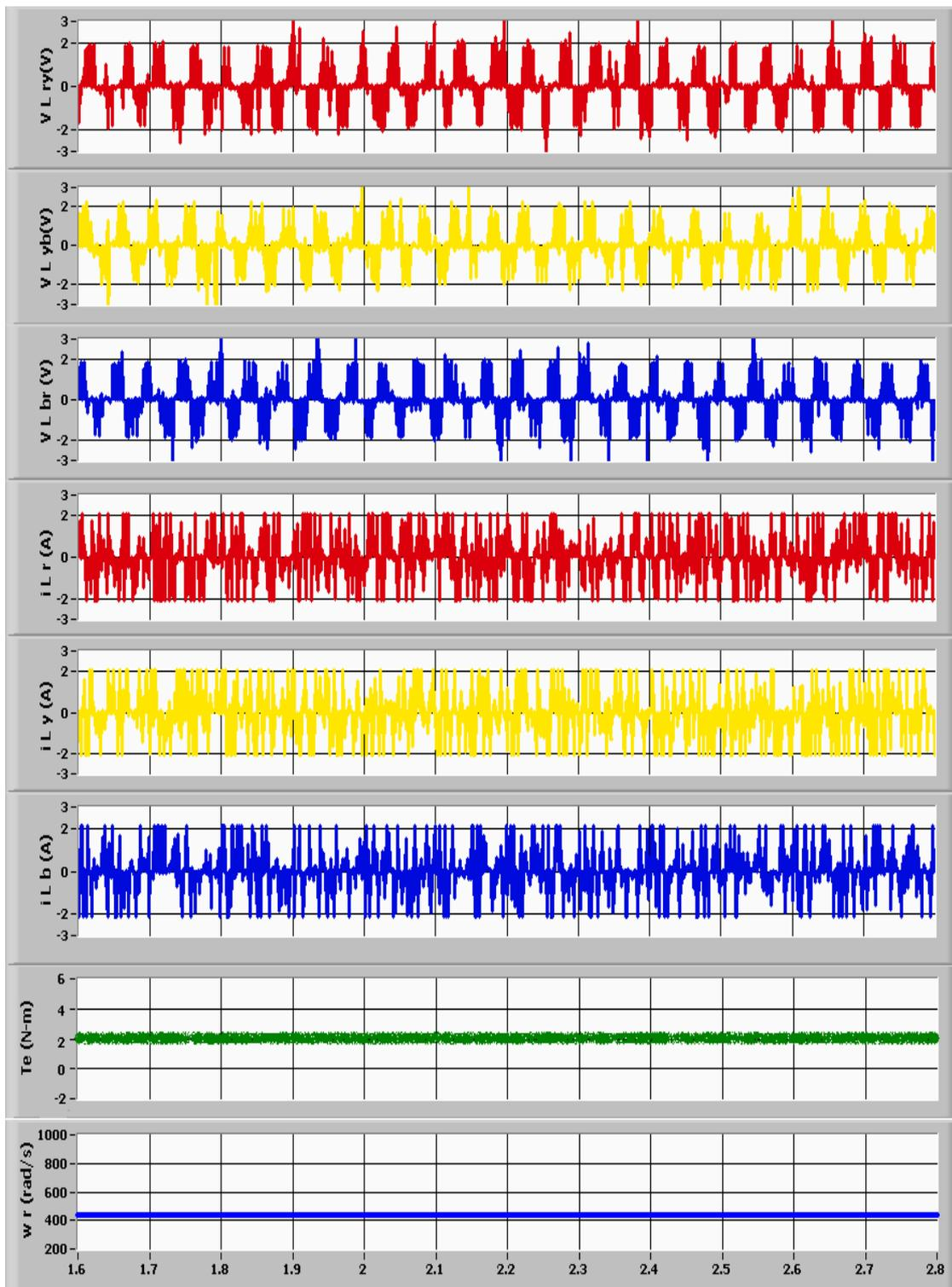
Figure 6. Experimental results showing three phase stator voltages, three-phase stator currents electromagnetic torque and rotor speed during SLG fault without providing any ride-through. Stator voltage scale: 100 V per division. Load current scale: 10 A per division. Electromagnetic Torque scale: 1 N-m per division. Rotor Speed scale: 1 rad/s per division.
