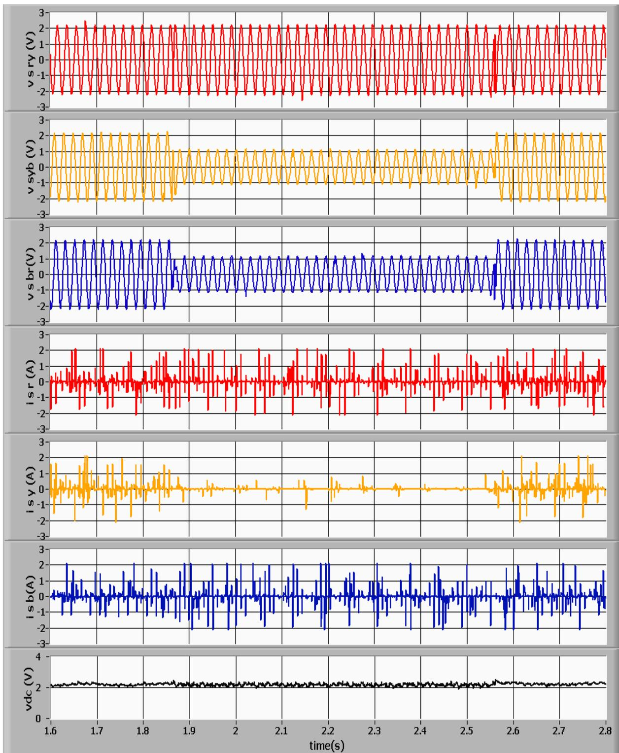
Figure 4. Experimental Results showing three-phase source voltages, currents and DC-Link voltage during SLG fault (Type-B) without any ride-through. Voltage scale: 100 V per division. Current scale: 2.25 A per division. DC-Link Voltage scale: 100 V per division.
