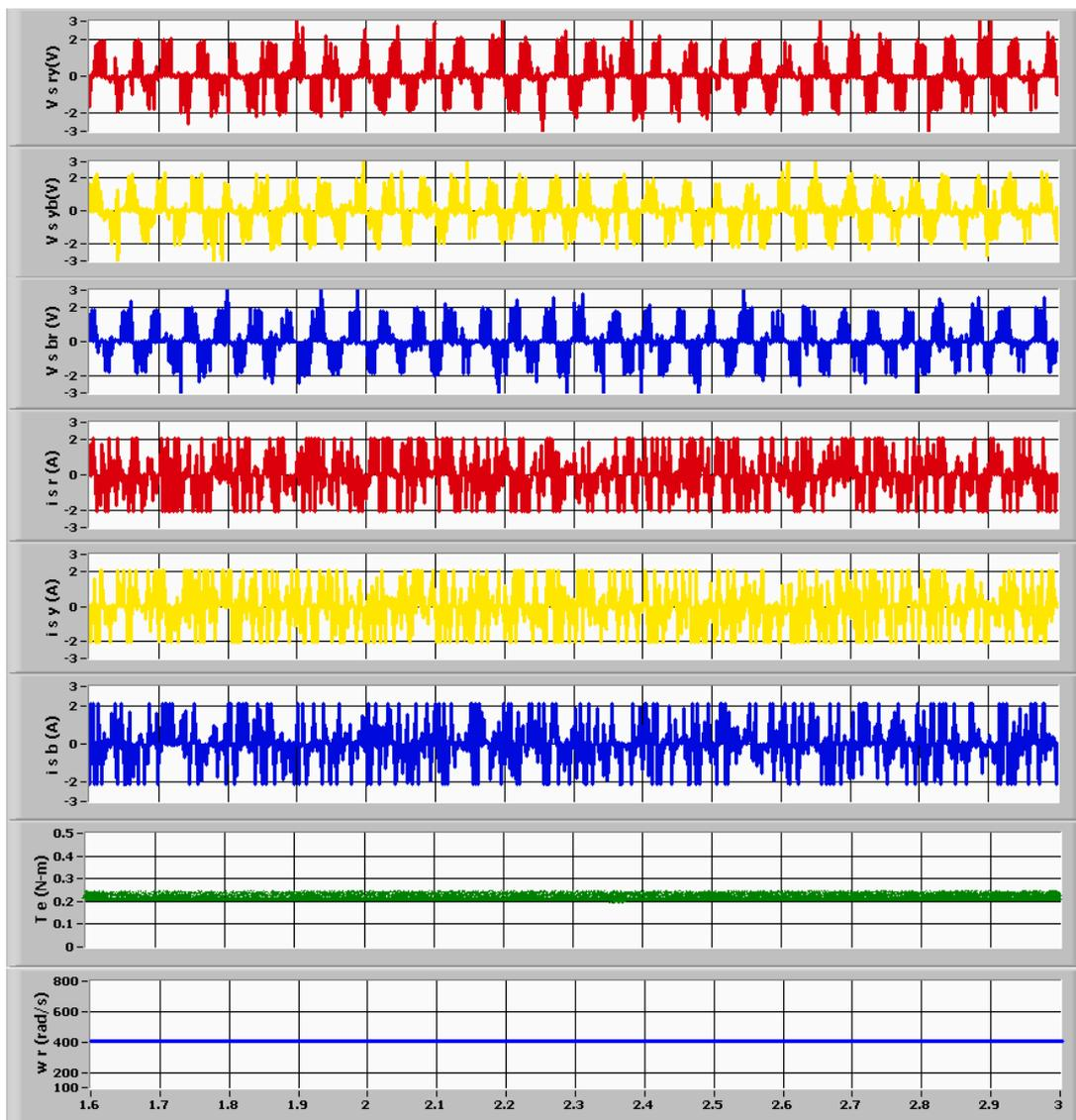
Figure 10. Experimental results showing three phase stator voltages, three-phase stator currents, electromagnetic torque and rotor speed during SLG fault (Type-B) with supercapacitor as ride-through alternative. Stator voltage scale: 100 V per division. Load current scale: 10 A per division. Electromagnetic Torque scale: 1 N-m per division. Rotor Speed scale: 1 rad/s per division.
