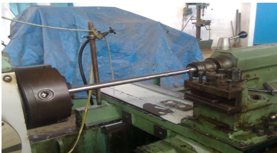
Figure 2: Set up of work piece on HMT lathe
