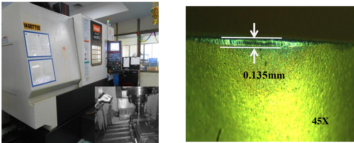
Figure -2: Mazak VMC and cutting zone Figure-3- Tool wear for 4 th Experiment
