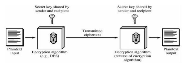
Figure 3: Data Encryption Standard
