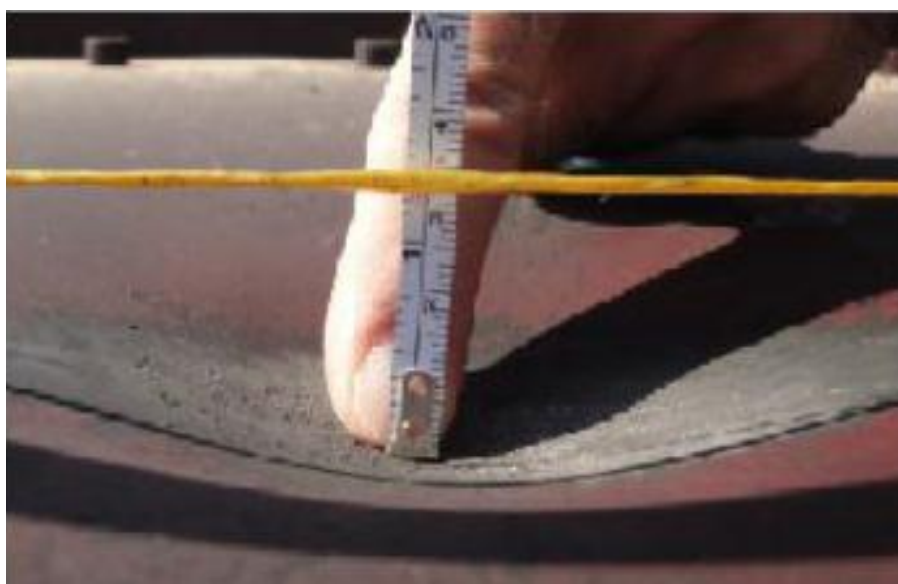
Figure 8: Measurement of created central deformation in scaled- down case
