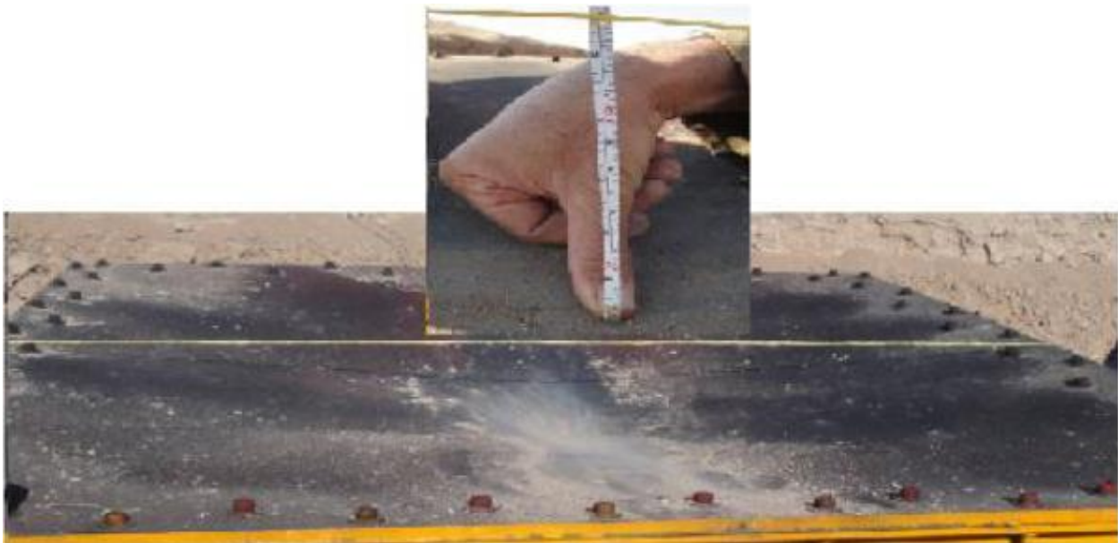
Figure 9: Measurement of created central deformation in full- scale case
