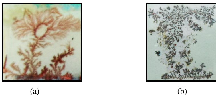
Figure:3 (a). Showing electro-less deposits with broken amorphous fragments
