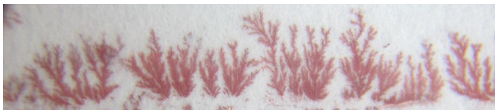
Figure: 2 (b). Showing electro-less deposition obtained with a 1 molar \text{CuSO}_4 solution in 8 hours
