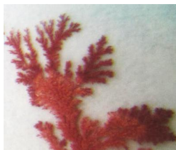
Figure: 2 (a). Showing lumps formation of copper metal deposits along with dendritic patterns
