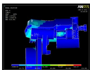
Figure 34. Bending of caliper.
