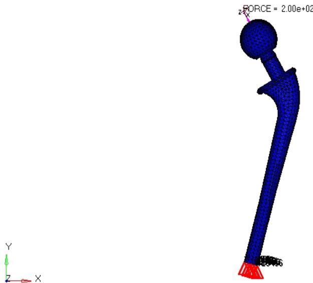
Fig 16. Model with Boundary Condition
