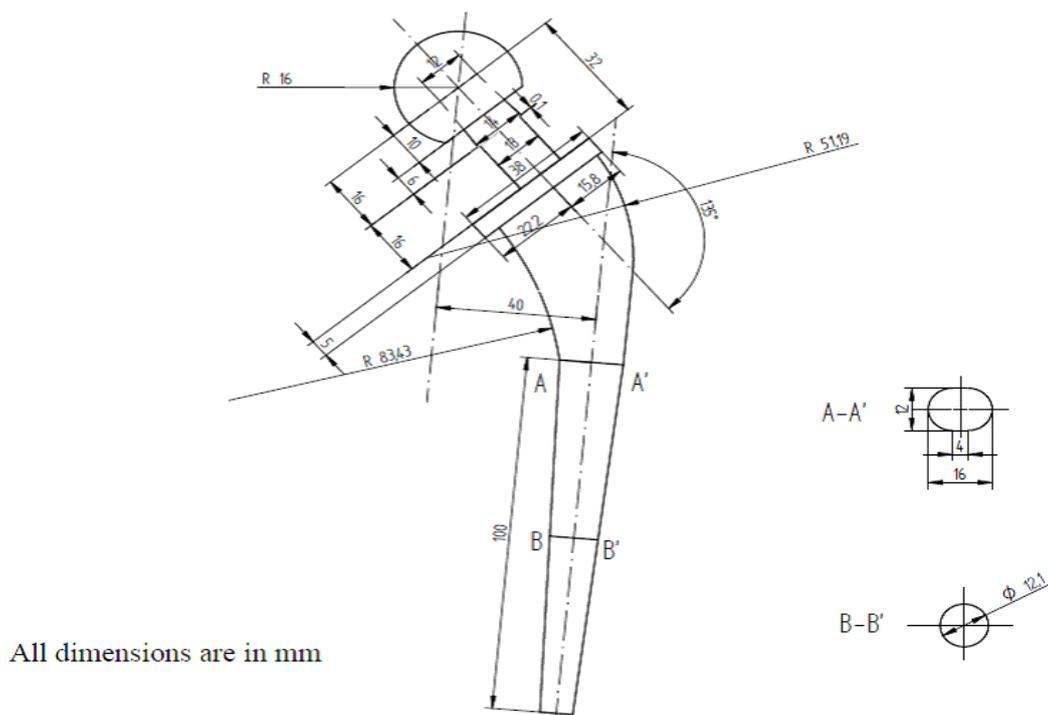
Fig.6. Geometry of the hip prosthesis
