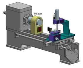
Figure 3. Heat resistance furnace with ultrasonic assisted equipment.
