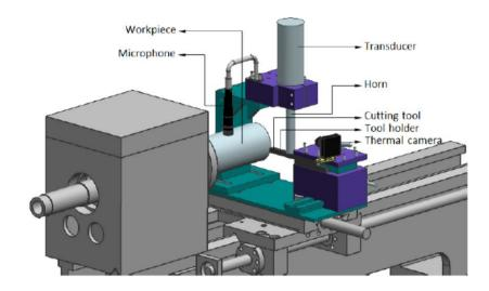
Figure 2.Ultrasonic assisted machining set-up
