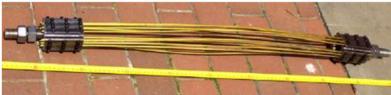
Figure 12. The SMA damper made up of 12 CuAlBe 3.4 mm diameter wires [17]
