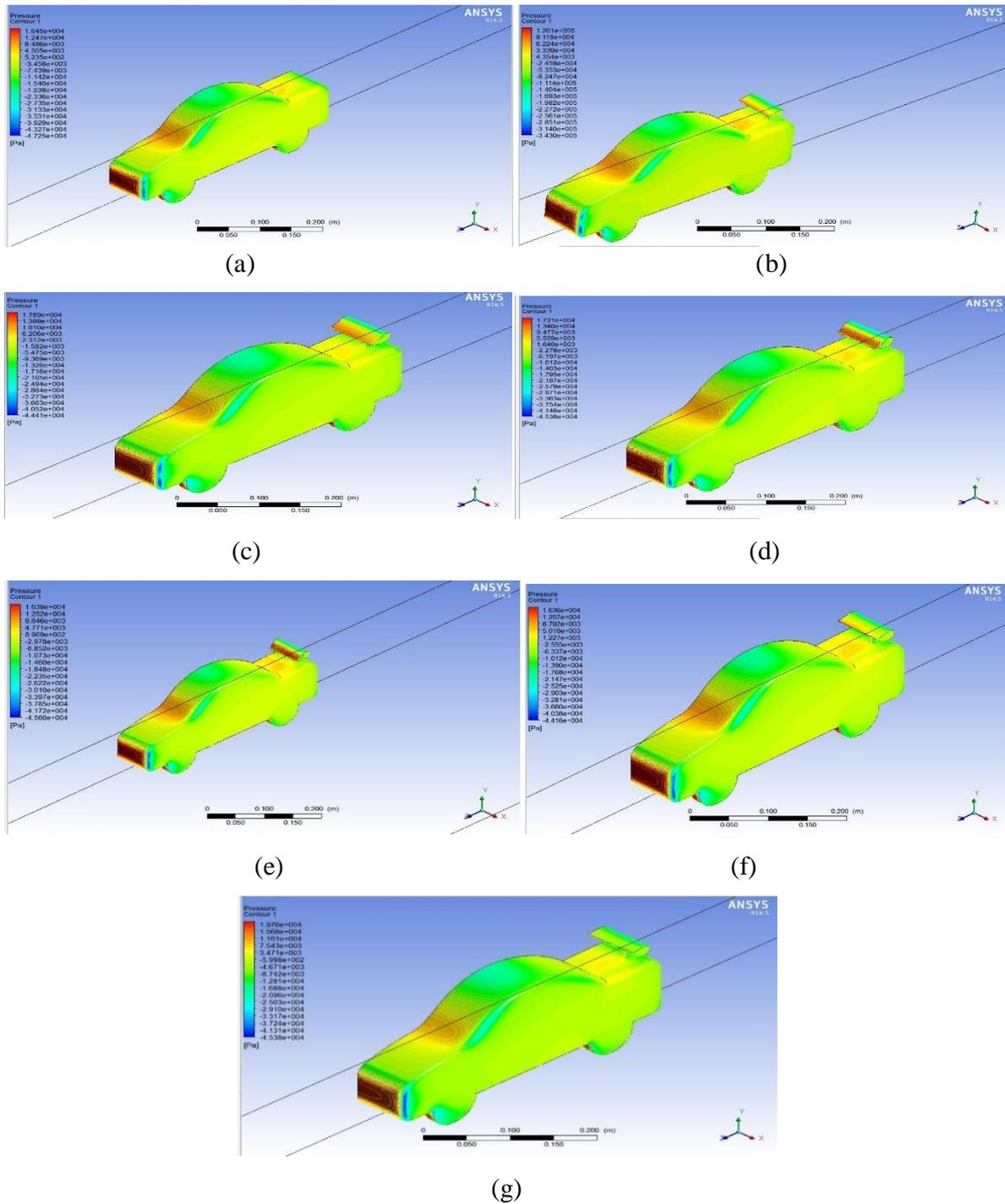
Figure 3. pressure contours over the car at 60 kmph with (a) without spoiler, (b) zero-degree spoiler, (c) ten-degree inclination spoiler downwards, (d) twenty-degree inclination spoiler downwards, (e) thirty-degree inclination spoiler downwards, (f) ten-degree inclination spoiler upwards (g) twenty degree inclination spoiler upwards.
