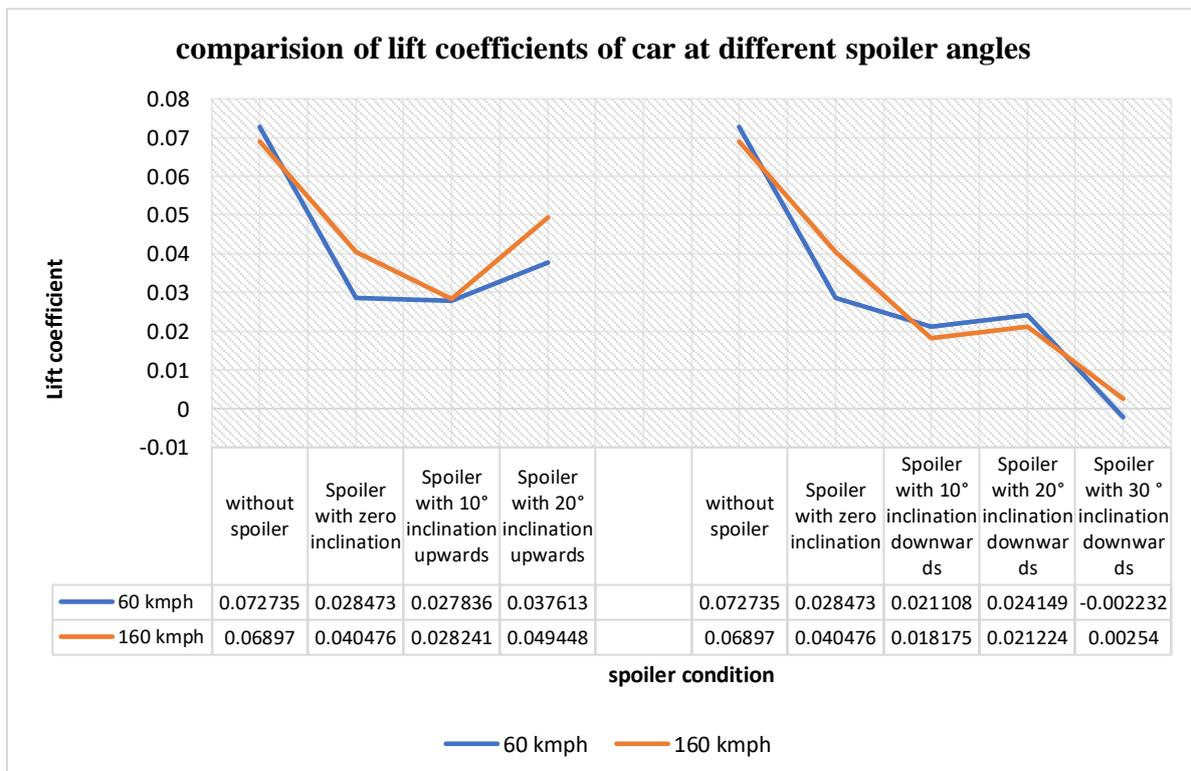
Figure. 7. comparison of lift coefficient of car at different velocities with varying spoiler angles.
