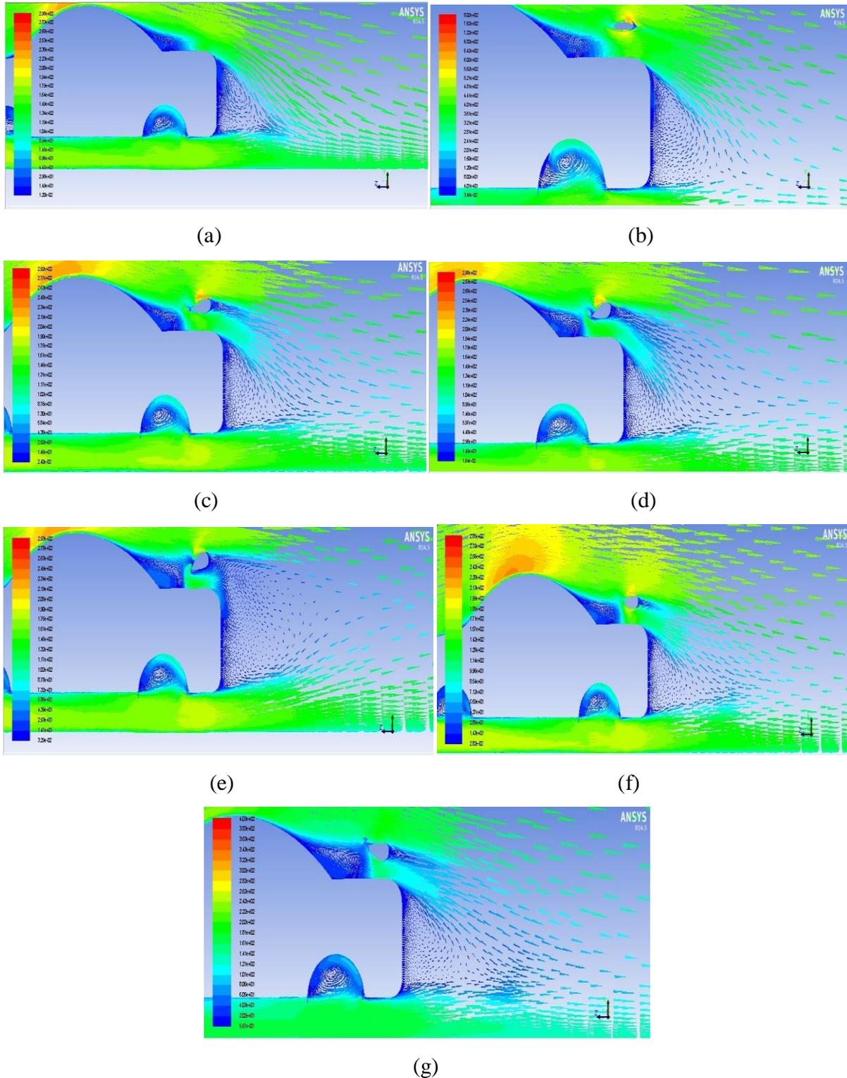
Figure 2. Recirculation zones at the rear end of car at 60 kmph (a) without spoiler (b) spoiler at 0 degrees (c) spoiler at 10 degrees downwards (d) spoiler with 20 degrees downwards (e) spoiler with 30 degrees downwards (f) spoiler with 10 degrees upwards (g) spoiler with 20 degrees upwards
