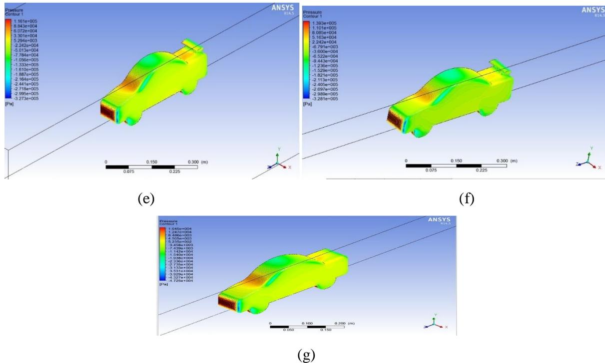
Figure 5. pressure contours over the car at 160 kmph with (a) zero-degree spoiler (b) ten-degree inclination spoiler downwards (c) twenty-degree inclination spoiler downwards (d) thirty-degree inclination spoiler downwards (e) ten degree inclination spoiler upwards (f) twenty degree inclination spoiler upwards (g) without spoiler
