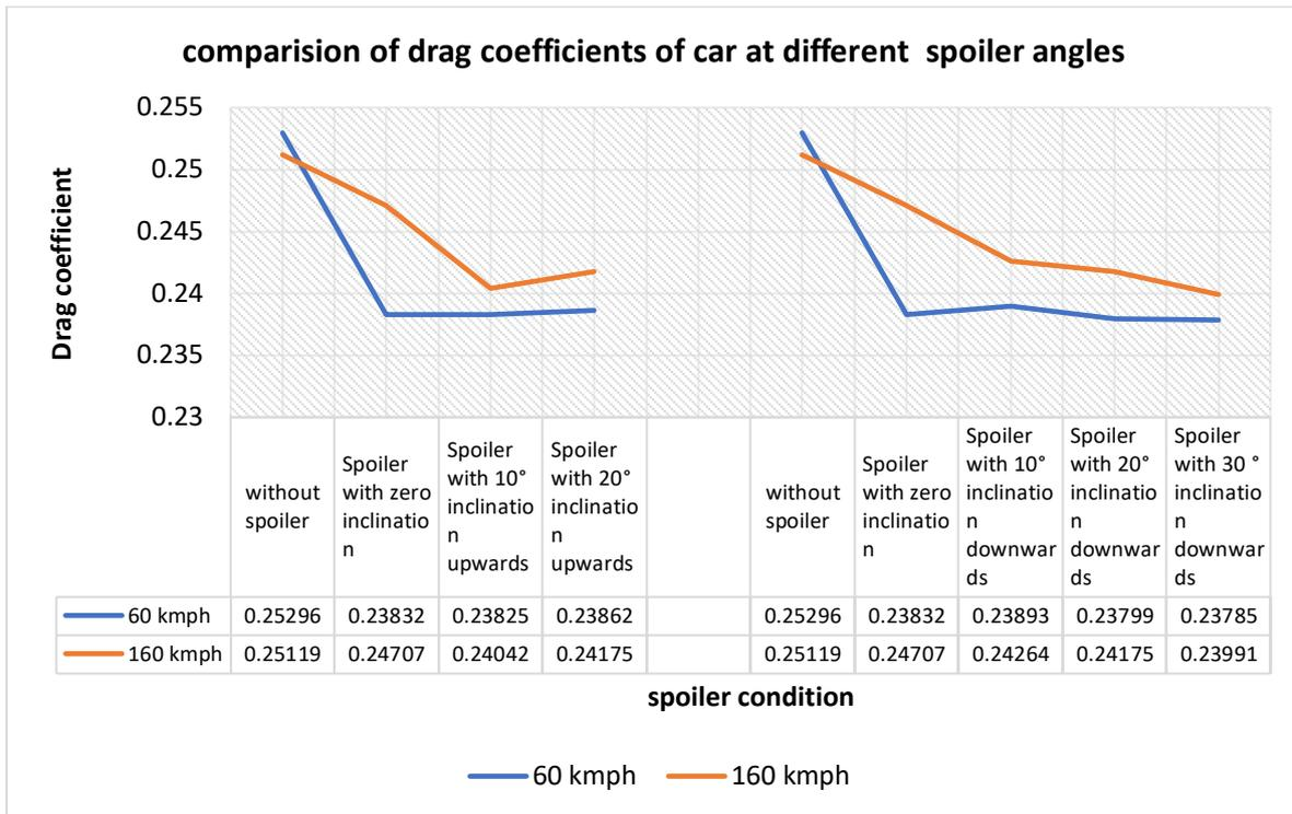
Figure. 6. comparison of drag coefficient of car at different velocities with varying spoiler angles.
