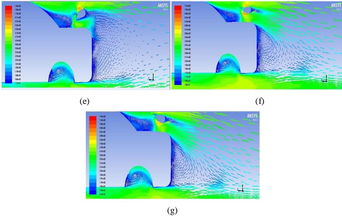
Figure 4. Recirculation zones at the rear end of car at 160 kmph (a) without spoiler (b) spoiler at 0 degrees (c) spoiler at 10 degrees downwards (d) spoiler with 20 degrees downwards (e) spoiler with 30 degrees downwards (f) spoiler with 10 degrees upwards (g) spoiler with 20 degrees upwards
