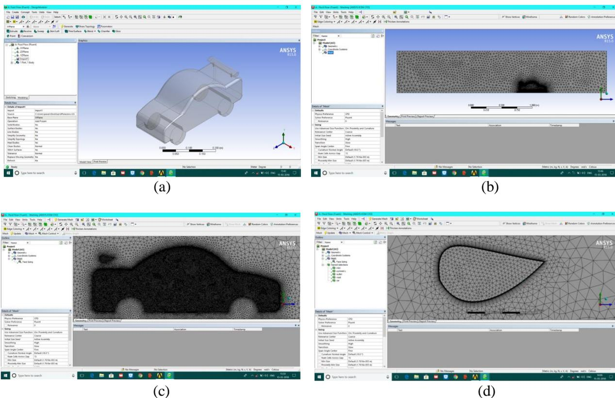
Figure 1. (a) Geometry of car, (b) Meshing of wind tunnel and car body, (c) Face sizing applied to car body, (d) Mesh showing inflation layer around the car body
