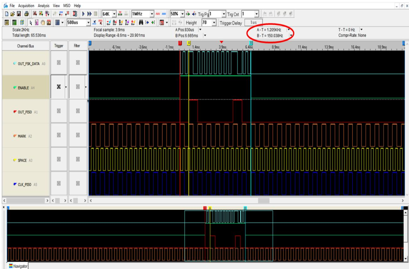
Fig. 19 – Testing of the system with the logic state analyzer sending the ASCII character "B" to the system (01000010)
