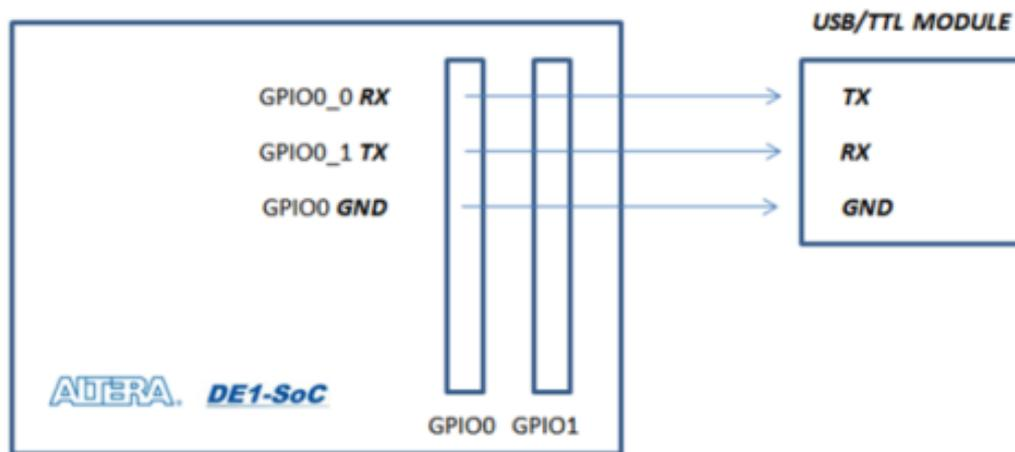
Fig. 16 - Connection scheme between the DE1\_SoC and the USB-TTL converter
