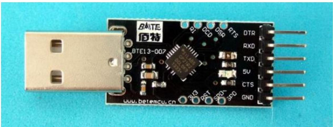
Fig. 15 - USB-TTL converter
