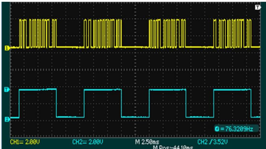
Fig. 23 - Time analysis of the FSK output and Enable output with sending to the system of the ASCII string "BCDE" (01000010- 01000011-01000100-01000101)
