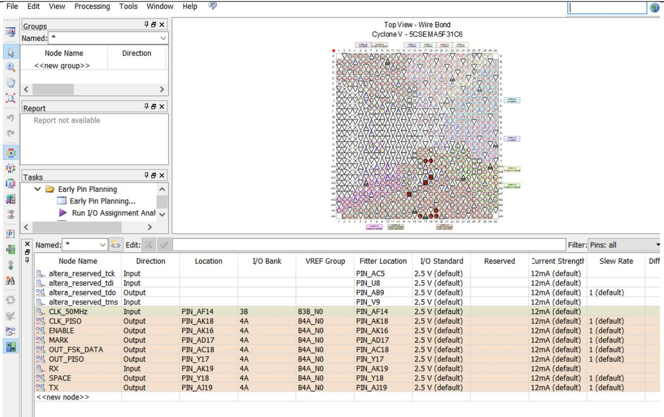
Fig. 14 - Pin assignment by using the Pin Planner tool in Quartus
