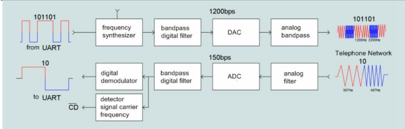
Fig. 2-Functional diagram of a UART-to-BELL202 converter
