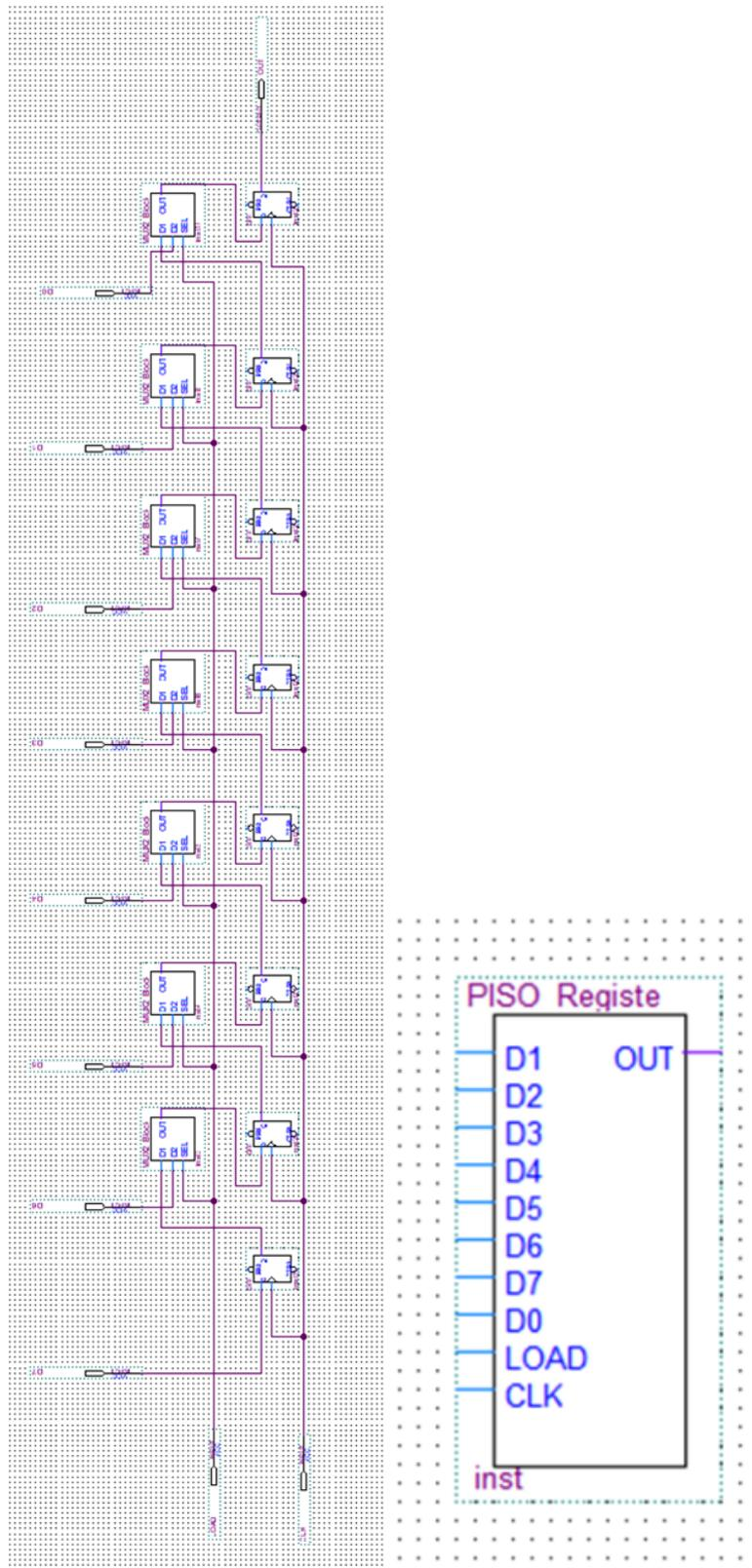
Fig. 7 – PISO register schematic and related symbol
