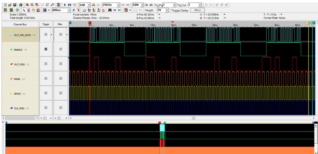
Figure 21 - Detection with logic state analyzers of the system functions by sending the ASCII string "BCDE" to the system (01000010- 01000011-01000100-01000101)
