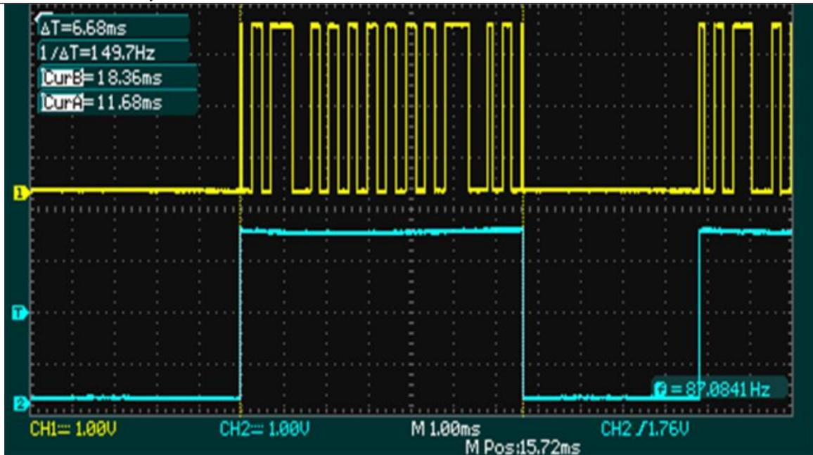
Fig. 20 - Time analysis of the FSK output and Enable output by sending to the system the ASCII character "B" (01000010)
