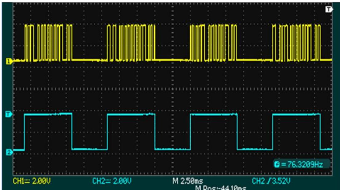
Fig. 23 - Time analysis of the FSK output and Enable output with sending to the system of the ASCII string "BCDE" (01000010- 01000011-01000100-0100010)
