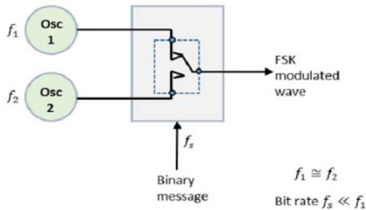
Fig. 3 - FSK modulator without phase continuity
