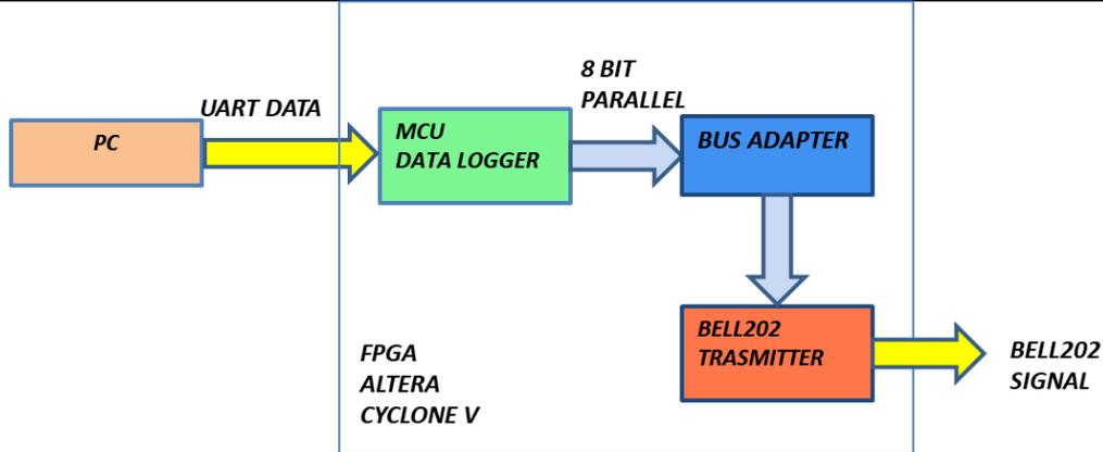
Fig. 4- Block diagram of the project
