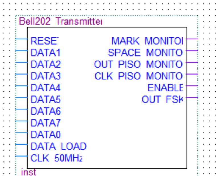
Fig. 6 - Transmitter circuit symbol
