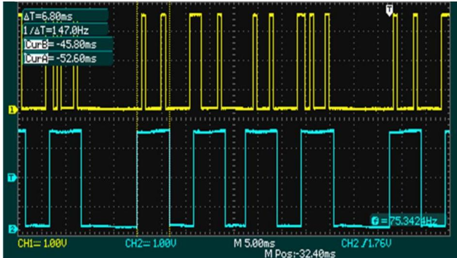
Fig. 22 - Time analysis of the FSK output and Enable output with sending to the system of the ASCII string "BCDE" (01000010- 01000011-01000100-01000101)
