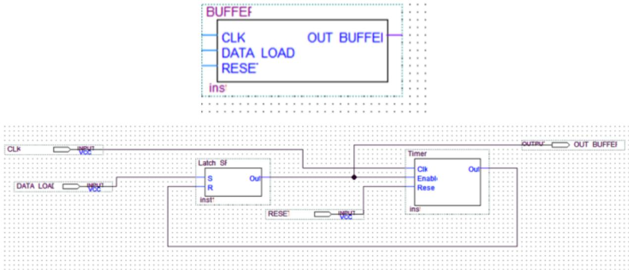
Fig. 9 – Buffer\_OUT schematic and symbol file
