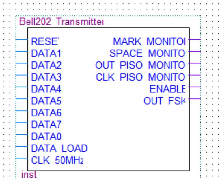
Fig. 6 - Transmitter circuit symbol
