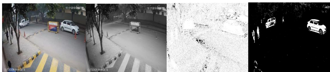
Figure 5 (a, b, c and d). The process of background subtraction in an image using frame differencing.
