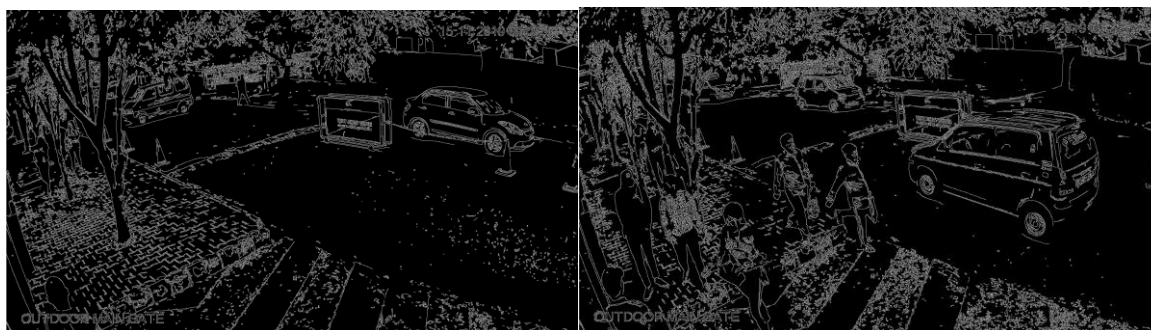
Figure 7. Images after background subtraction using Canny Edge detection
