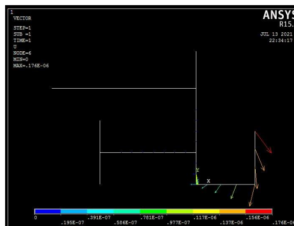
Figure 3. The Displacement contour of the Hook
